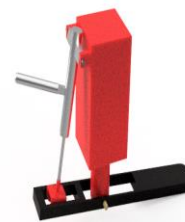
Figure 5: Dummy of the concept In the above figure, the 3d model of the concept is shown. The linear actuator produces a moment about the elbow that lifts the wrist end. The actuator can either be attached at the back of the elbow or ahead of the wrist. Mounting it either ways will bear not much significant effect on the effectiveness of the actuator. The bill of materials required to build the actual model would be as follows:
