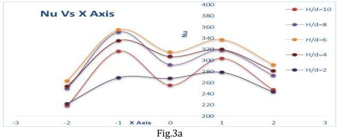
From Fig 3a it is For H/d ratio 6 maximum heat transfer takes place ,then for H/d ratio 4 ,8.It is Surprising to note that least heat transfer takes place at H/d ratio 2.Also at Point of Impingement for all H/d ratio heat transfer is less. At the farther end from impinged point heat transfer is very less. For Y/d ratio of 1,-1 there is increase in heat transfer.
