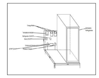
Fig.3, 3D cad model of test rig on domestic refrigerator
