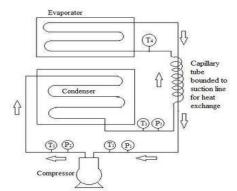
Fig. 1, Layout of Refrigeration system [6]
