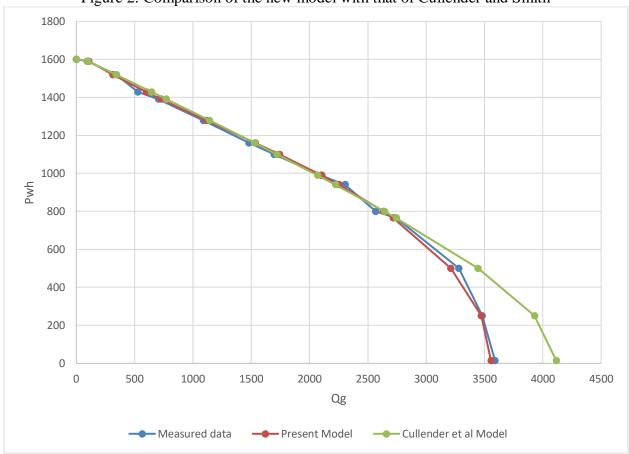
Figure 3: Comparison of the new model with measured field data and Cullender et al model.
