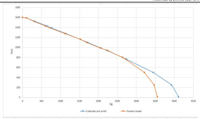
Figure 2: Comparison of the new model with that of Cullender and Smith
