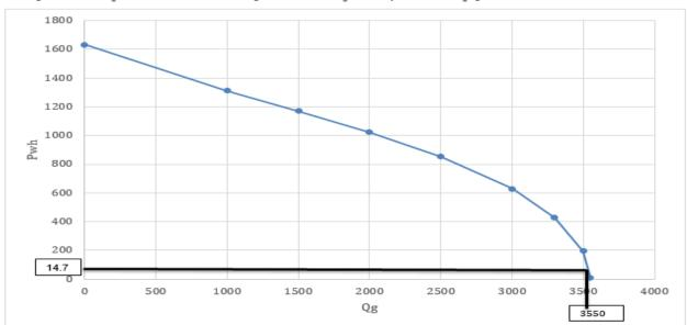
Figure 1. Wellhead Pressure – Gas Production rate Curve generated for the well. The Absolute open flow of the well evaluated at pressure of 14.70psia is **3550 MMSCFD.**
