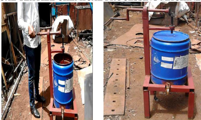
Figure 2. Fabricated Manual Textile chemical mixing and processing machine
