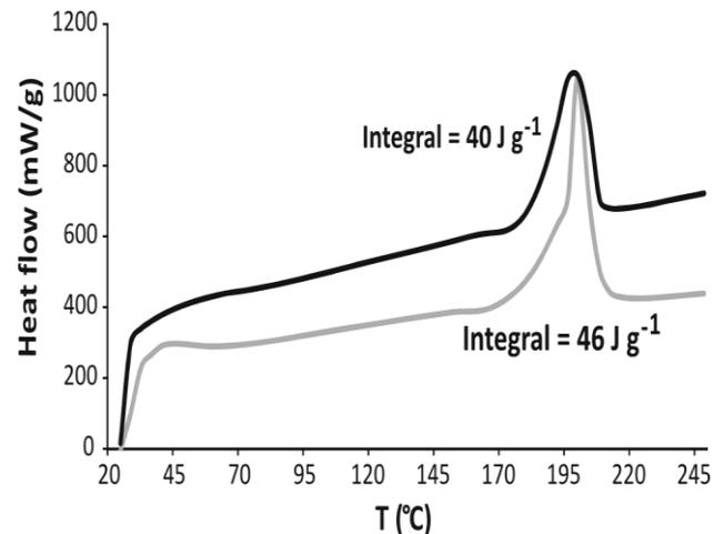
Fig. 3 First heating curves of the DSC measurements for samples made of the nylon copolymer printed at air (gray) and under a nitrogen atmosphere (black)
