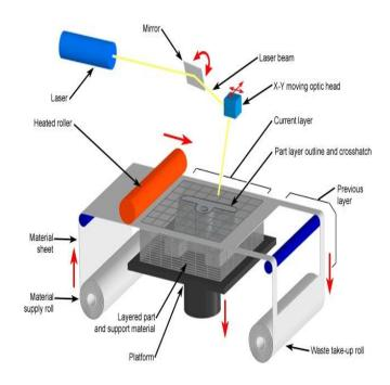
Fig. 6. Laminated Object Manufacturing
