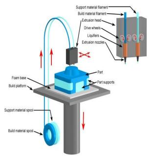
Fig. 4. Fused deposition modeling
