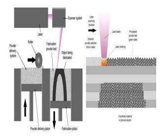
Fig. 3. Selective laser sintering
