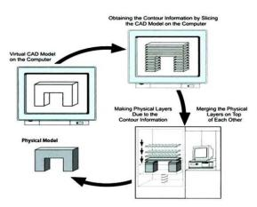
Fig. 2. Printing procedure
