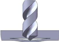
Fig. 1. Delamination mechanism
