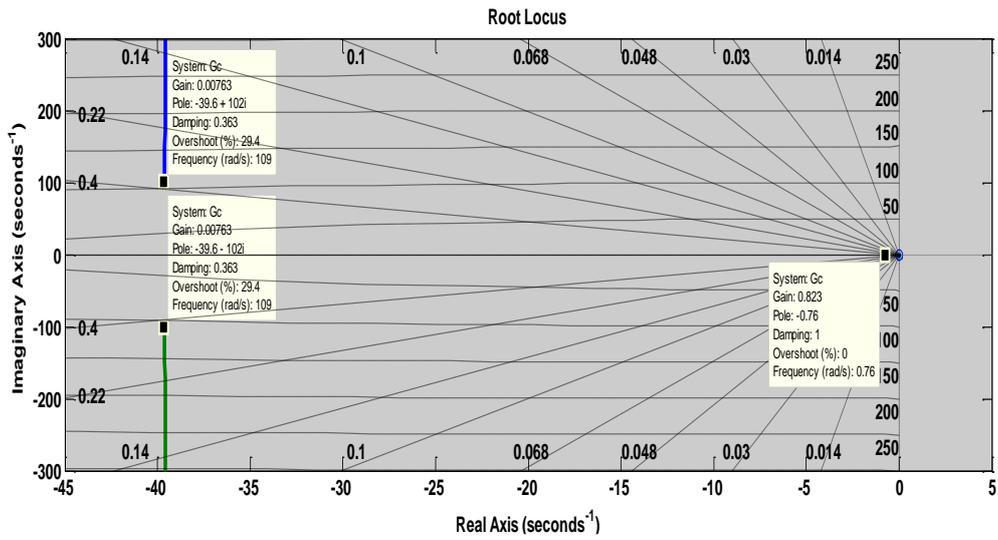
**Fig 5: Root Locus of Closed-Loop System using a PID Controller.**
