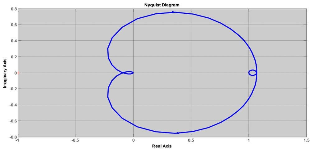
**Fig 6: Nyquist plot using a PID controller**
