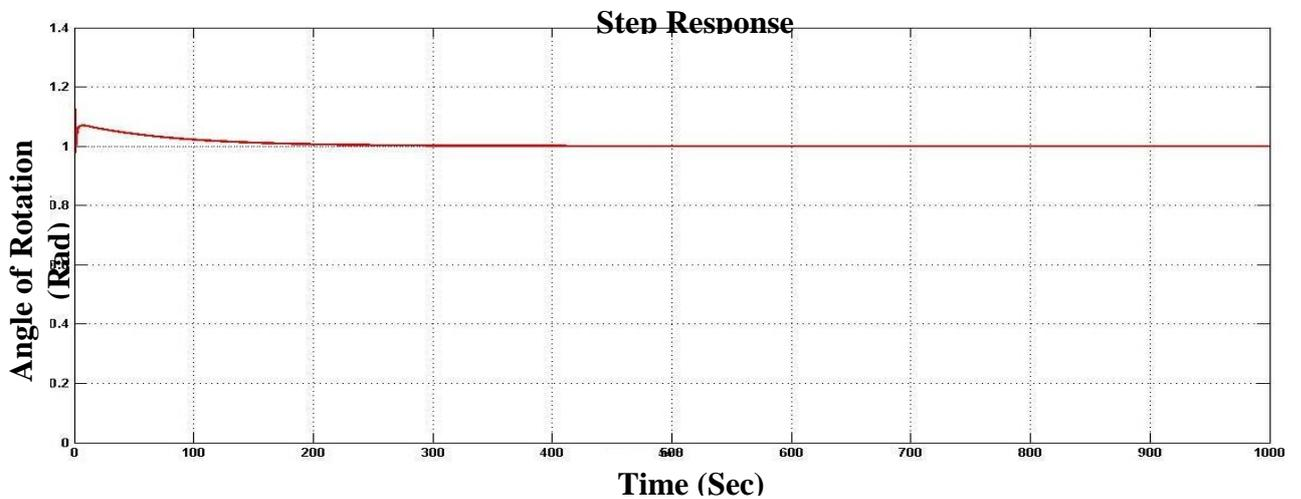
**Fig.4: Step Response after using a PID Controller.**
