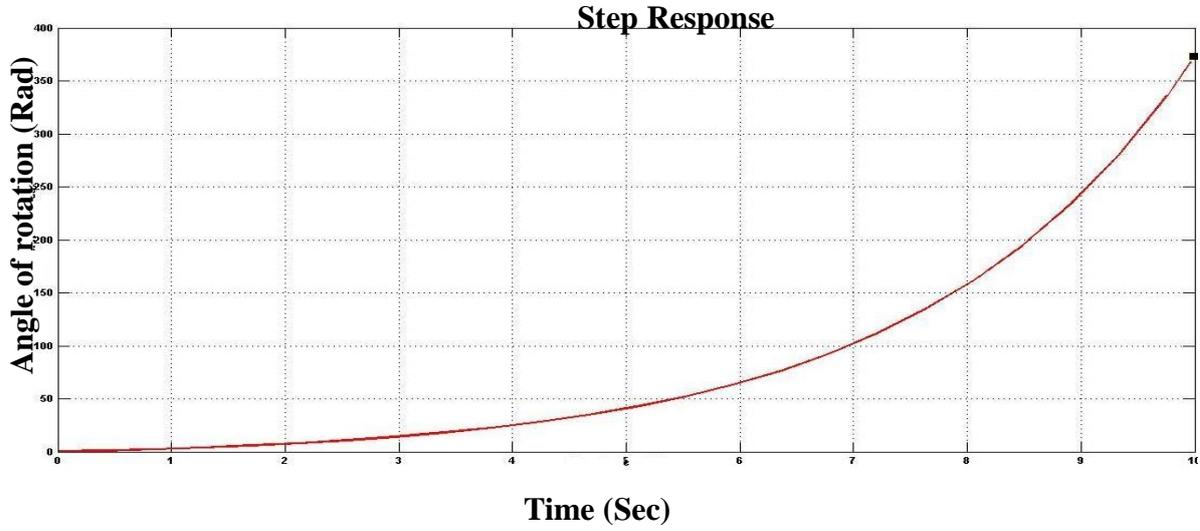
**Fig 2: Open Loop Step Response of the Single Joint**
