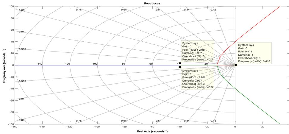
**Fig 3: Root-Locus of Open-Loop system with a Pole at Right half side of S-Plane**
