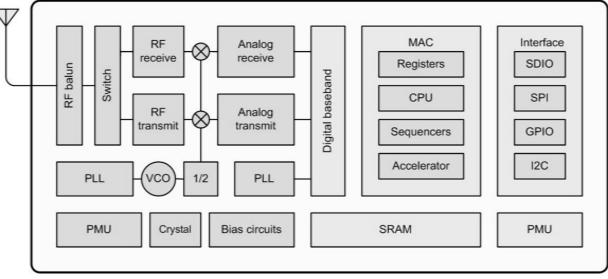
Fig.3: Block Diagram of IOT Module
