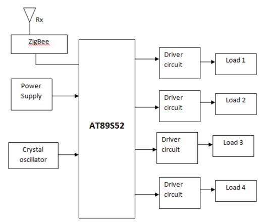
Fig.2: Block Diagram of Embedded System
