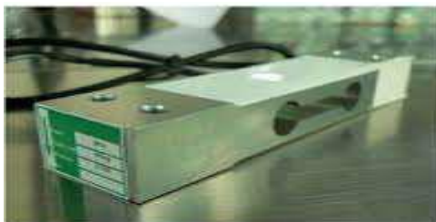
Fig.2: Cantilever type load cell(CEL 601)
