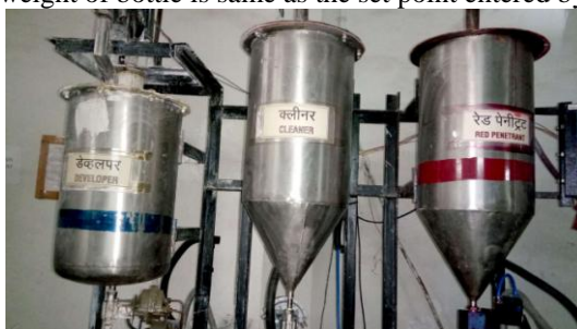
Fig.5: Tanks with solenoid valve
