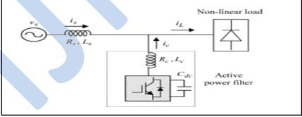
Fig. 1. Shunt Active Power Filter Working Principle
