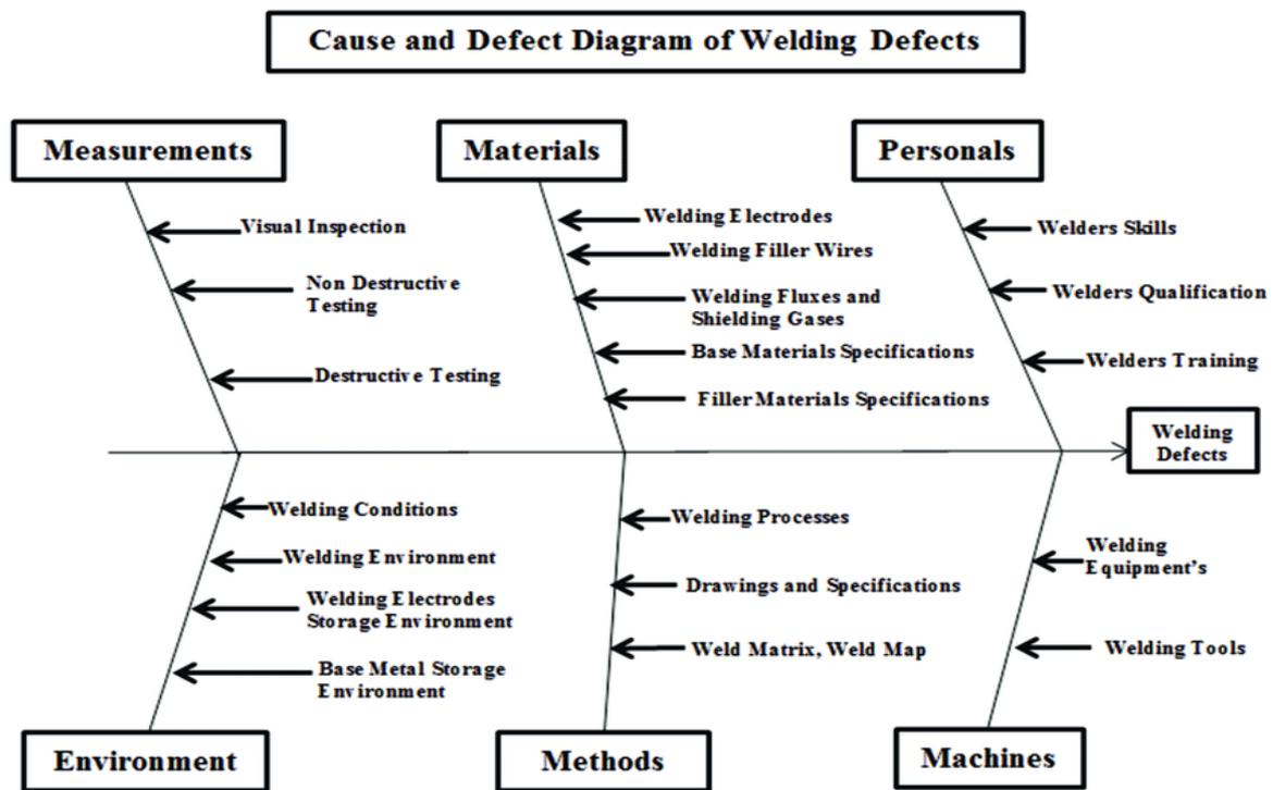
Fig.1 Cause effect diagram for welded joint
