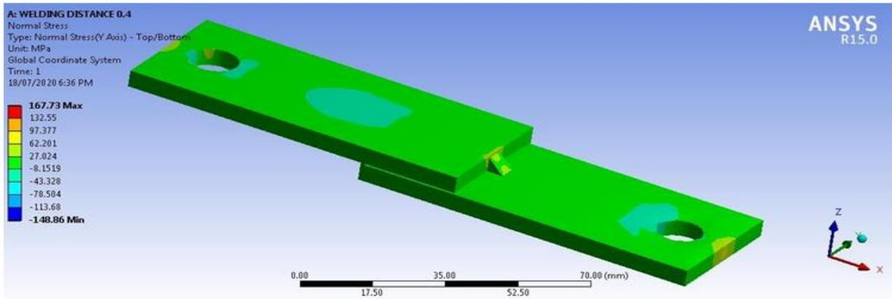
Fig.31 Simulation of workpiece 7
