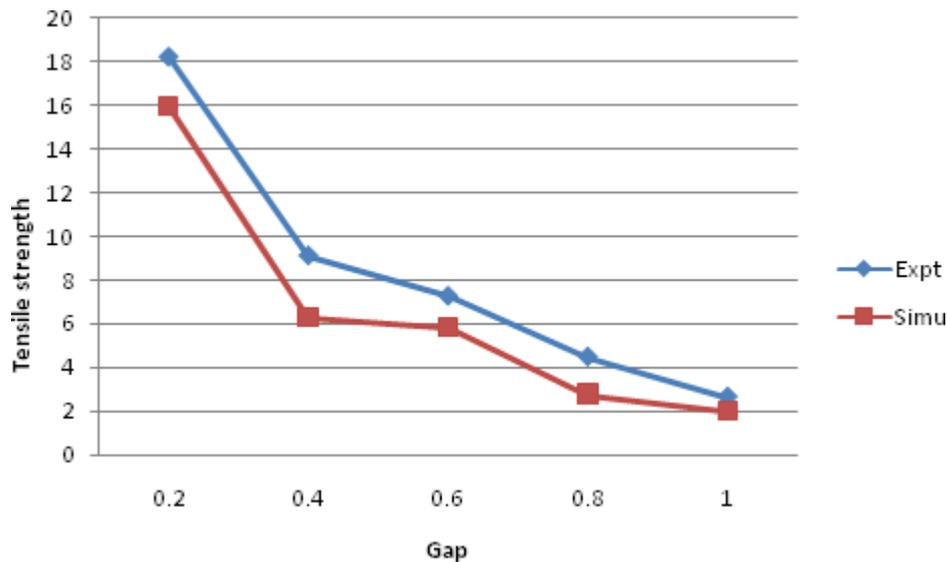
Fig.41 Difference between experimental and simulation result
