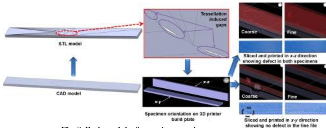
Fig.8 Cad model of gap size specimen
