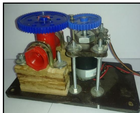
Figure 3.2: DC motor operated valve
