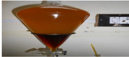
Fig.4.5 Separation of methyl ester and glycerine of vegetable oil.
