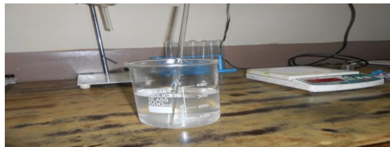
Fig. 4.2 Sodium Methoxide solutions for Transesterification process
