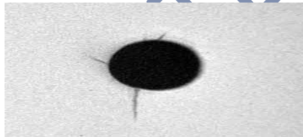
Cracks & Cold shuts
