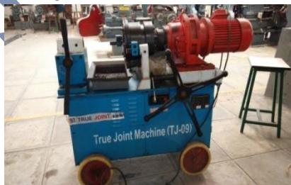
Figure 2: True joint (TJ-09) machine
