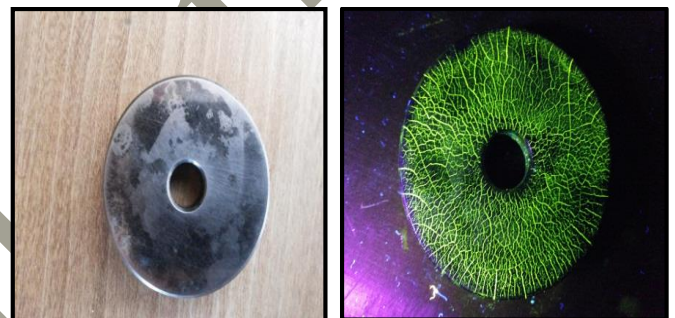
Fig 5 Image of component under simple and uv light
