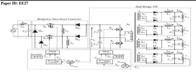
Fig 1-Circuit configuration of proposed multiple output switched mode power
