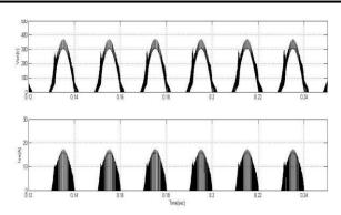
Fig 4 -Voltage across Switch Sp and Sn and Current through switches.
