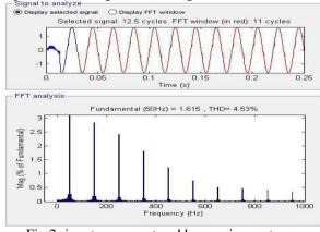
Fig 2- input ac current and harmonic spectrum
