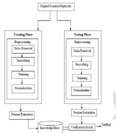
Figure 1: System Architecture
