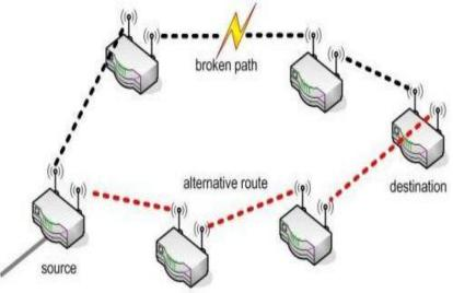
Ability of self-healing in a wireless mesh network
