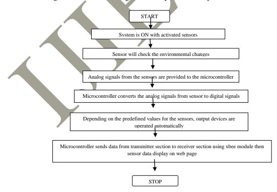
Fig. 3. Flow chart of the execution steps for the proposed system
