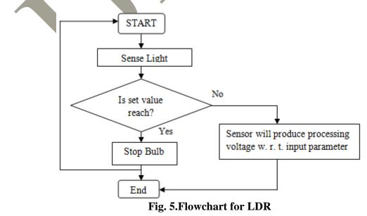
An LDR is made of semiconductor material Cadmium Sulphide (CdS). The light falling on the brown zigzag lines on the sensor causes the resistance of the device to fall. This is known as a negative co-efficient. Since LDR is extremely sensitive in visible light range, it is well suited for the proposed application. In this system, when the Light rises to 70 lux, system will switch off bulb in the proposed system.
