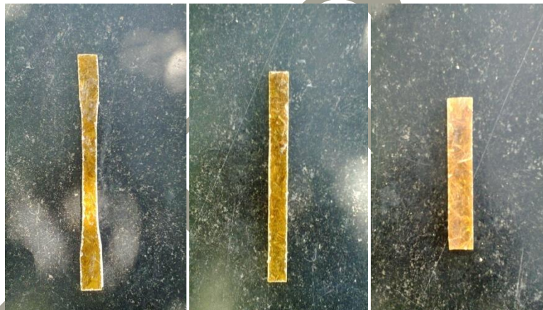
Fig.2.4: shows tensile specimen, flexural specimen, impact specimen after cutting to desired specimen from Wire Hacksaw
