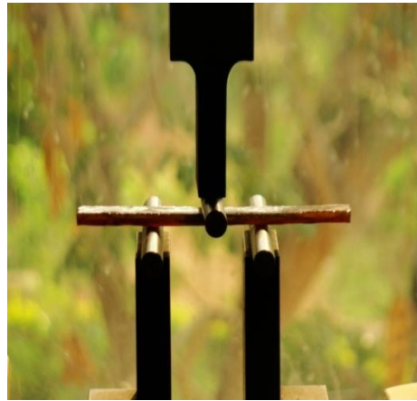
Fig 3.2: Specimen undergoing flexural test
