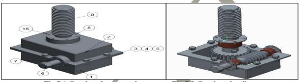
Fig 7.1 Gearbox for manual system Fig 7.2 Gearbox details
