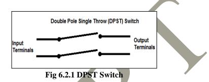
Each terminals of a double pole single switch can be in the (closed) or in the off (open) condition .A Double Pole Single Switch has a lot of versatility or the variation being that it accepts 2 inputs, which makes it able to drive 2 different outputs in a circuit. It drives depends on the circuit design and what the circuit is intended to do. But DPST have enormous applications in circuits.
