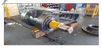
Fig 1.1 Jaw Placed on the Wooden Blocks
