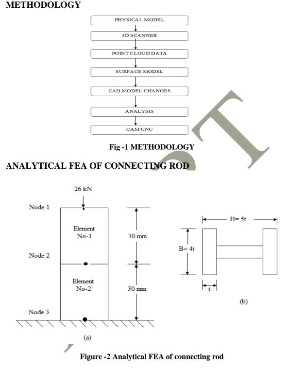
$\label{eq:matrix} \begin{array}{l} \mbox{Material-20CrMo alloy steel} \\ \mbox{Modulus of Elasticity E=210 GPa = 200 x 103 MPa} \\ \mbox{$\rho$=7800 kg/m3 = 76518 \times 10 -9 N / mm3$} \\ \mbox{Cross sectional area=} 2 \times 4t \times t + 3t \times t = \\ 11t2 = 11 \times 152 = 2475 mm2$ \\ \mbox{Elemental stiffness matrix} \\ \mbox{For element no1} \\ \mbox{$F2$} = (A \ 1 \ \rho)/2$ \end{array}$
