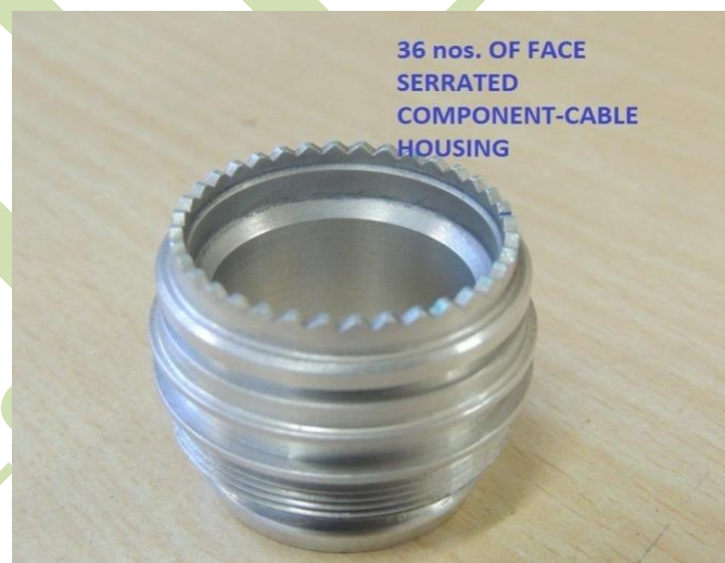
Figure 1: Cable Housing have face serration
