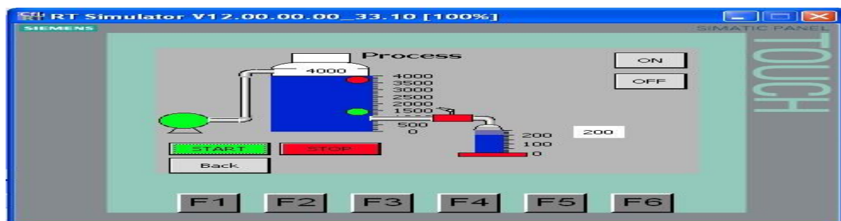
Fig 5 Pump ON tank filled completely in TIA
