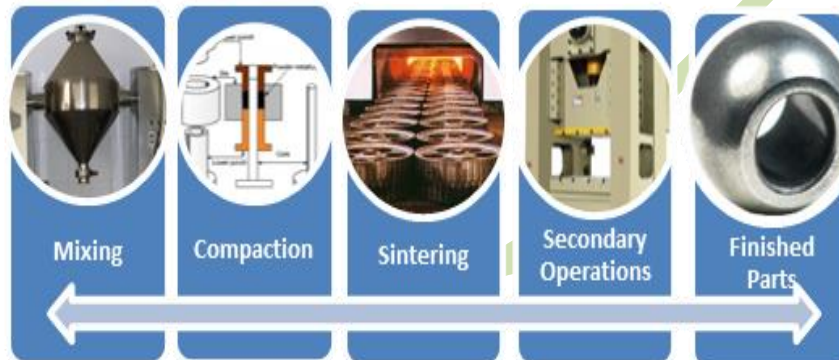
Figure 1. Manufacturing Process of Sintered Parts
