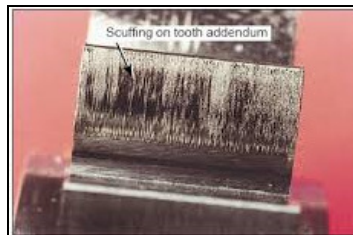
Fig.2- Scuffing on tip of gear tooth
