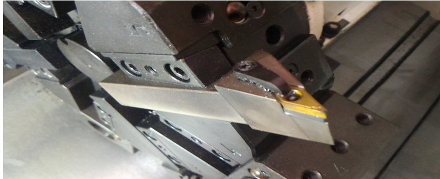
Figure 2: Rhombus Shape Insert Used For Turning Operation
