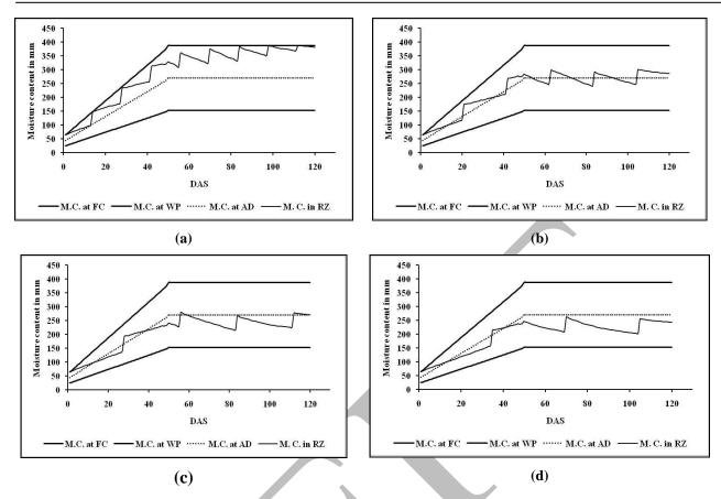
Figure 1. Variations in moisture content of root zone of wheat at (a) 14 days interval and 70 mm depth (b) 21 days interval and 70 mm depth, (c) 28 days interval and 70 mm depth and (d) 35 days interval and 70 mm depth
