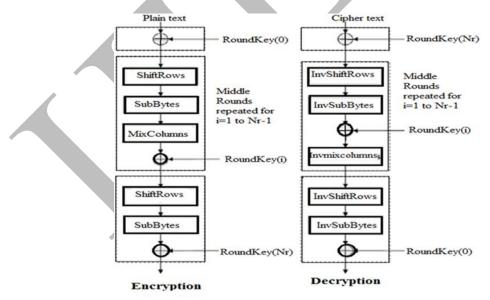
Fig.2: AES Encryption and Decryption data flow.
