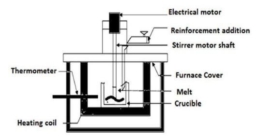
Fig 1 Schematic view of stir casting setup [7].
