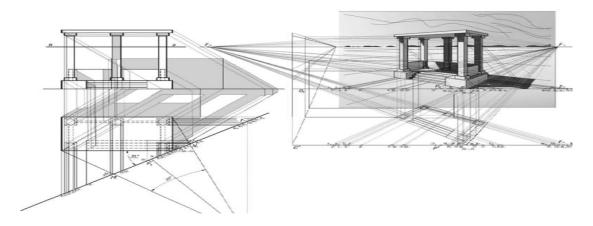
To construct the shadow of a curve line, it is enough to construct the falling shadows of a number of points belonging to this line and connect them with a smooth curve.
