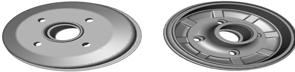
Fig.1 Typical Automobile Brake Cast Iron Drum
