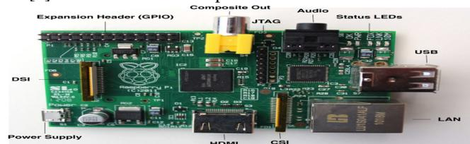
**Figure 2 : Front side of Raspberry Pi**
