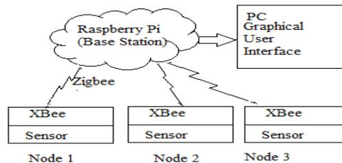
**Figure 1 : System Monitoring Architecture**
