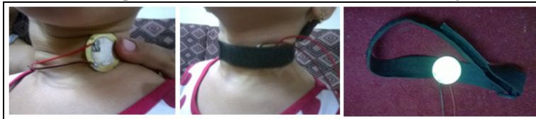
Figure 4: During the speech production, the microphone must be in direct contact with the lowest part of the speaker's throat, with a reasonable but comfortable pressure.
