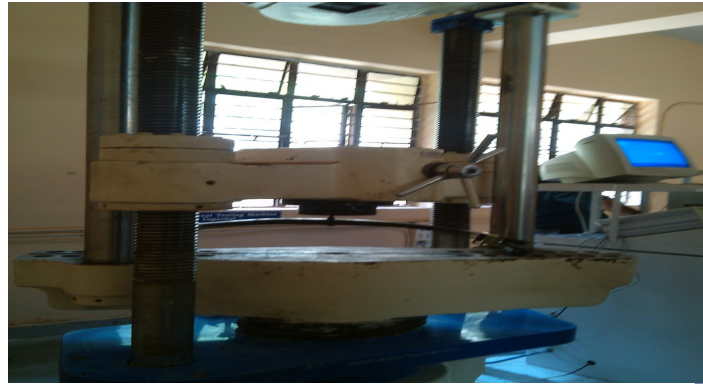
Figure 2: Testing of conventional leaf spring on UTM machine
