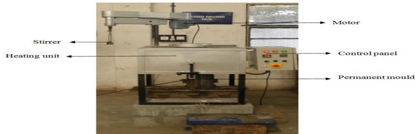
Fig 3.1 photograph showing experimental set up for the stir casting
