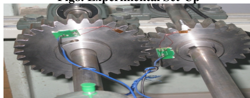
Fig9. Strain Gauges Applied on Gear Teeth Face
