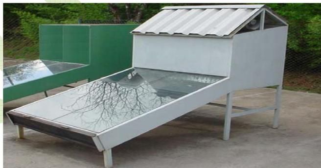
**Fig: Hybrid solar-electrical dryer**
