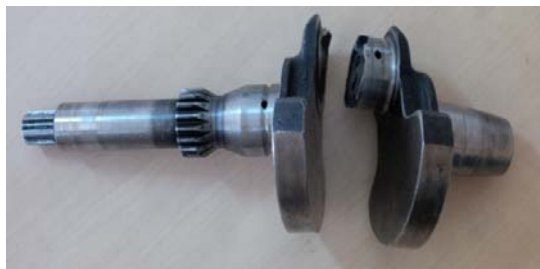
Fig. 1 Final failure on fillet of crankshaft
