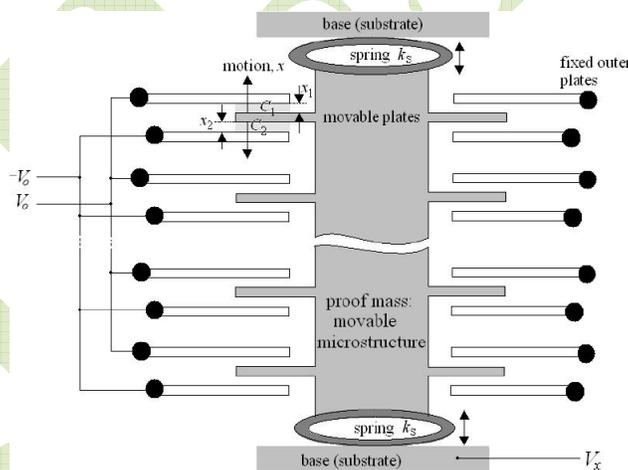
Fig 2.MEMS Accelometer
