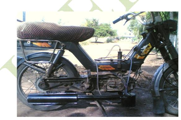
**Fig: Fabricated Turbocharger With Engine Arrangement**
