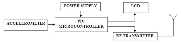
Fig.2.1. Block Diagram of RF Transmitter section
