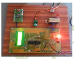
Fig. 4.1. Hardware of Transmitter Unit
