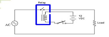
Fig.3.4 Relay Circuit
