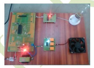
Fig. 4.4. Hardware of Receiver Unit (Light OFF and Fan OFF)
