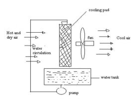
The present evaporative coolers use a cooling media made wet by water flow. Hot and dry air is made to flow over this media with the help of a fan or blower. The water in the cooling media gets evaporated due to heat of air. Thus the temp of air reduces and water vapour formed, mixes with air. The relative humidity of air increases. Normally 5-10°c reduction in the temp of air is possible.
