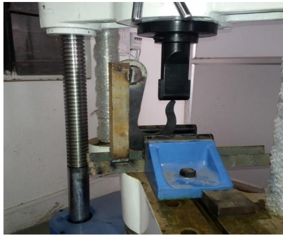
Fig. 10. Experimental testing of hook on UTM
