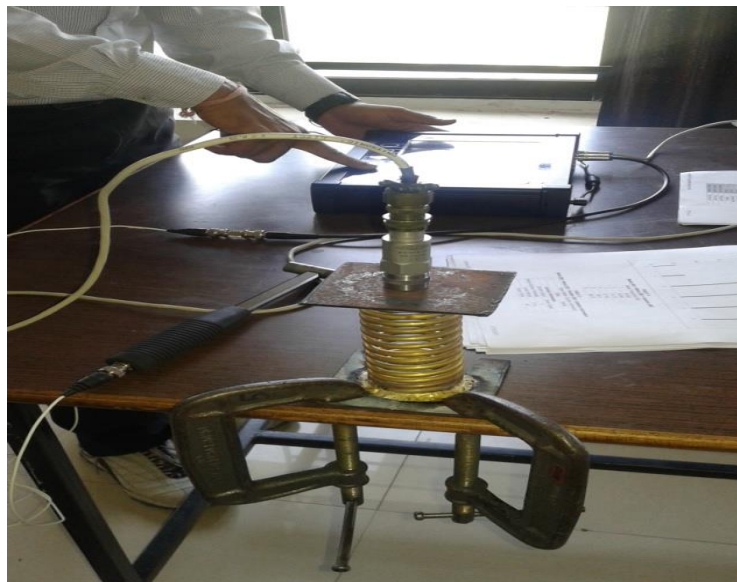
Fig. 8 Experimental setup for Brass spring
