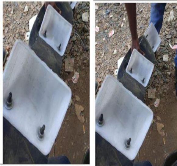
Fig.6 Belt Bucket Conveyor
