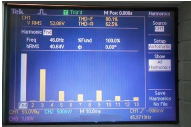
Fig. Harmonics generated by 3-level Inverter across resistive load
